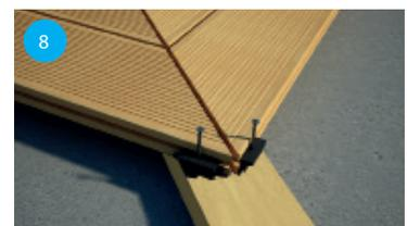
When fitting two boards at 90° ensure a minimum expansion gap of 5mm where the boards meet. Ensure hidden fixing clips are used at both board ends.
