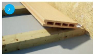
Tilt first deck board so that the leg of the deck locates underneath the lip of the perimeter starter clip.
