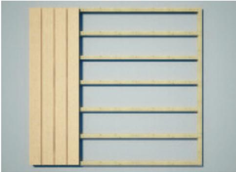
Each board should be supported by 3 joists. Ensure a slight fall of 2° to aid water run off.
